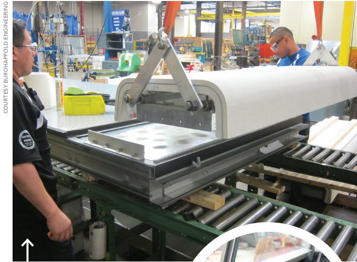
A piece of GFRG for the Vagelos Center at Columbia University being installed onto a unitized curtain wall panel at Permasteelisa's factory. Inset shows a base bracket for the glass fin.
