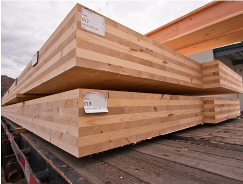
CLT is the basis of the tall wood movement, as the material's high strength, dimensional stability and rigidity allow it to be used in mid- and high-rise construction. Photo courtesy of Structurlam
