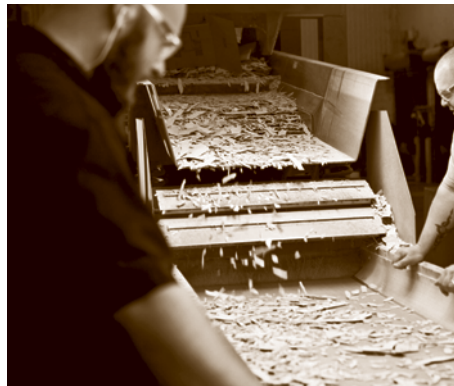
Following the 2010 Vancouver Olympics, Mannington Commercial took 200,000 square feet of vinyl graphic materials by 3M Canada (as shown in photo at left), diverted it from landfill, reprocessed the waste material at its Georgia production facility (center), and recycled it into commercial flooring material that was later installed in a school (right). More such case studies can be found at http://achievegreen.net/ .
