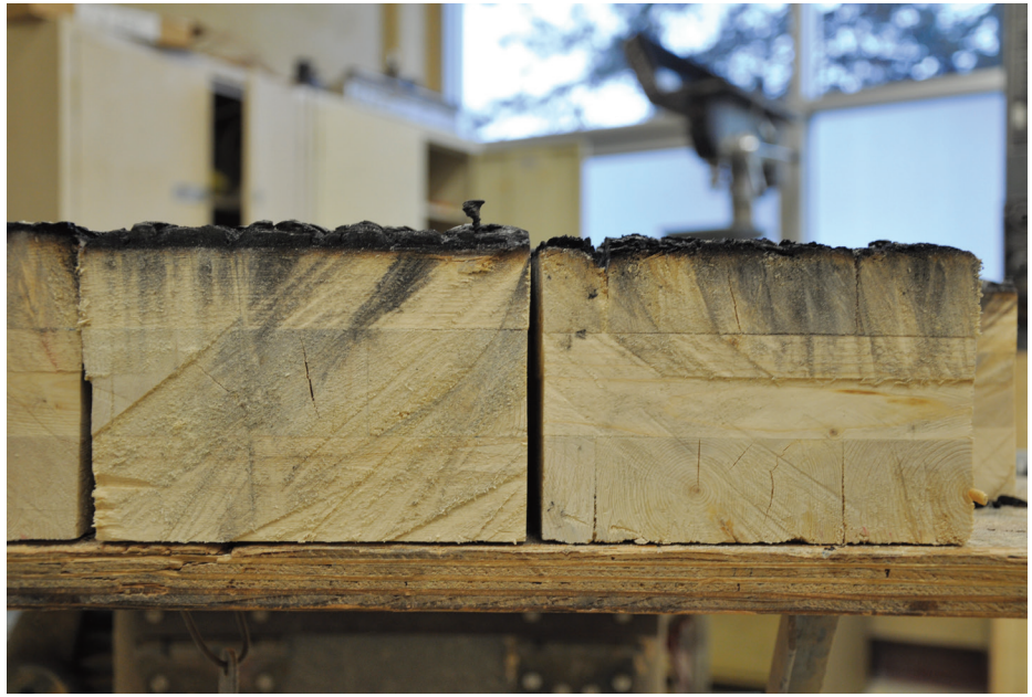
Fire tests show that CLT chars slowly at predictable rates.
