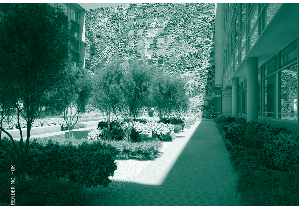
Water wall garden in the net-zero carbon office prototype. Vegetated walls along the east and west facades of the links between the office bars provide aesthetic continuity and moderate the outdoor climate. The south facade has an edible food garden area (not shown) as an additional amenity for building occupants.
